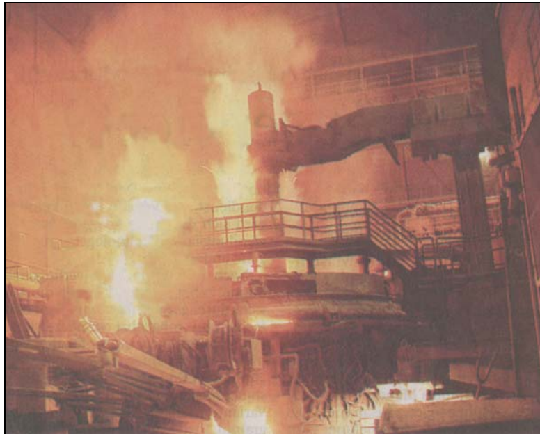
EAF in the melt shop of Peine Salzgitter melting Scrap with a graphite electrode with a diameter of 800 mm. Foto: SGL Carbon
